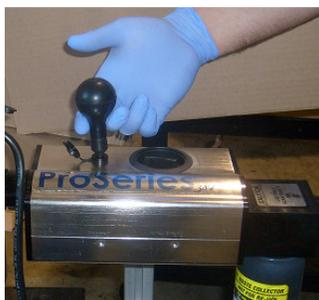
**Figure 1. Place purge bulb on to vent cap**
