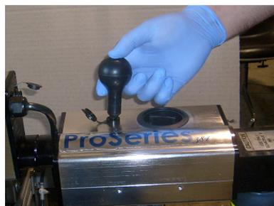
**Figure 2. Place thumb on top of purge bulb**
