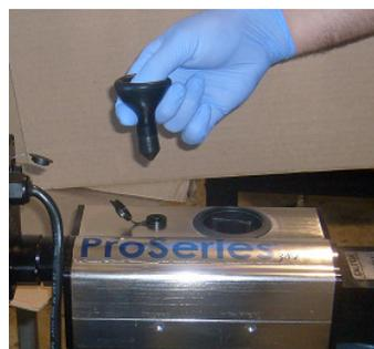
**Figure 4. While applying pressure remove bulb**
