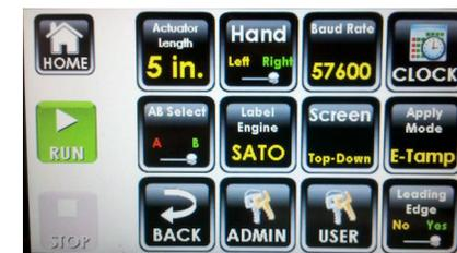
**ACTUATOR MOTOR** - Controls the direction and speed of the actuator with five (5) discrete speeds for label application to the product. MCM II monitors speeds of the actuator, stalls, and position of the actuator during travel.
