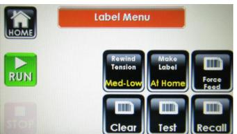
**Make Label** Determines the label generation mode. For slow applications, like pallets, make this **P1 Detect**. This will reduce the time the label adhesive is exposed to air and drying. For highest throughput, use **At Home**, for batch runs. User **P2 Detect** for the highest accuracy (by using two detectors) when print on demand is required
