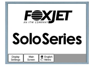
From the Startup Screen you can adjust the display's contrast and backlight brightness, select the units of measure used throughout the other screens, or proceed to the main operating screens. Once you exit the Startup Screen you cannot return except by cycling power to the Handheld Controller.
