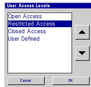
Controls within this box set the user access level. Buttons outside the box mirror the Home Screen and indicate which functions are password protected and which are open.
