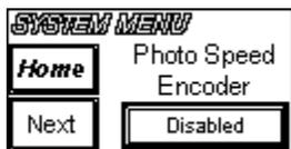
The Photo Speed Encoder is an optional device to measure the exact speed of the product as it passes the photosensors to provide the best match of label speed to the product speed. This results in better accuracy of label placement. Select Enabled if the Photo Speed Encoder is installed. By enabling this mode of operation, the Feed Speed Job Menu selection is replaced by Linespeed Encoder Offset.
