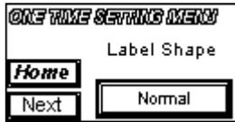
The Label Shape has two choices of Normal and Irregular. Normal should be used for rectangular opaque labels and Irregular should be used for round or non-rectangular shaped labels or when a registry mark (black mark) is used for clear labels. Irregular mode allows the system to end on a blank area of liner without interpreting this as a missing label.
