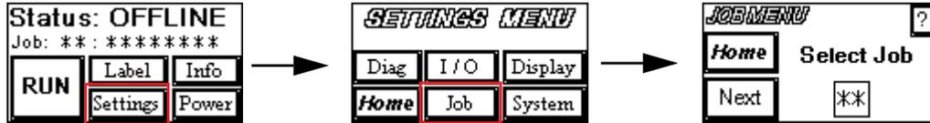
Beginning in the Offline mode, press the Settings button. From the Settings Menu, which can be passcode protected (default passcode from the factory is 9999), select the Job button choice. This enters the Job Menu selections. See section [Job Settings Screens on page 36](#) for information on how to make these selections.
