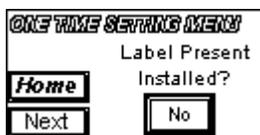
If the Label Present sensor is installed on the unit, press the button below the text until it displays "Yes".
