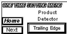
The selections are leading or trailing edge. By selecting leading edge, the label placement on the product is justified to the front or leading edge of the product. By selecting trailing edge, the label placement is justified to the back or trailing edge of the product.
