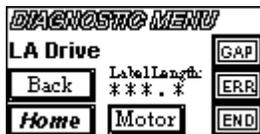
The Label Applicator Module Diagnostic screen tests the drive motor, motor shaft encoder, and the gap sensor. With the system webbed and calibrated, slide the label gap in and out of the gap sensor. View the gap signal on the display. Press the Motor button and the label will advance to the gap. At the end of the run, the approximate label length will be displayed. If the length displayed is incorrect or doesn't update, there could be a problem with the motor shaft encoder.
