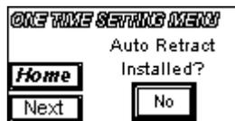
If the Auto Retract sensor is installed on the unit, press the button below the text until it displays "Yes".
