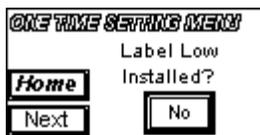
If the Label Low sensor is installed on the unit, press the button below the text until it displays "Yes".
