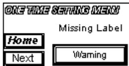
The system detects a missing label on the liner roll after each label feed. The system can allow the missing label, and advance to the next position when Missing Label is set to warning. This will display on the user interface and light the warning tower yellow. If Error is selected, the system will halt operation on a missing label.
