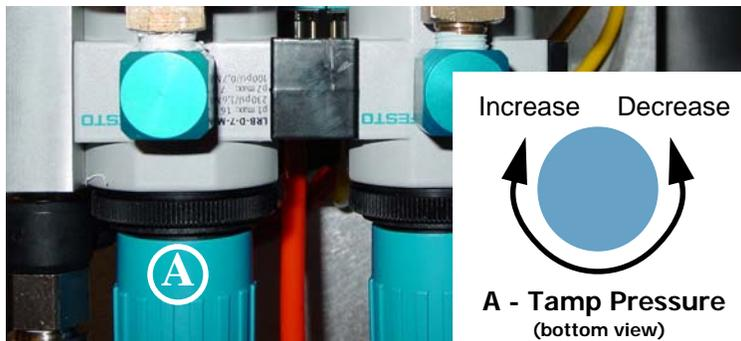
For applications requiring higher throughput, increase the pressure to a value between 50 - 70 psi. For light touch applications, reduce the pressure to a value between 30 - 40 psi.
