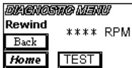
The Rewind Diagnostic screen will allow the user to test the motor by pressing the TEST button. This will activate the motor briefly, to verify operation and correct direction. The motor's RPM will be displayed to verify that the motor's feedback sensors are working as well.
