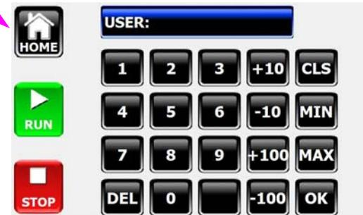
Can be set to up to 8 digits. If User Passcode is set to 0 the menus with user protection will be unprotected.
