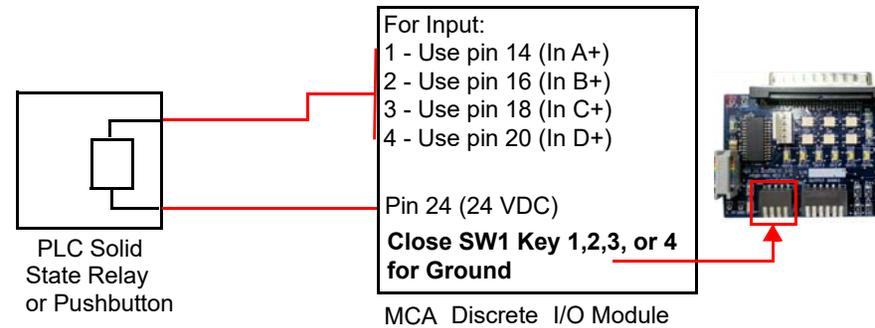
Connection to PLC triggering MCA input, PLC Sourcing Power
