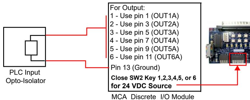
Connection to High Power Relay from MCA Output
