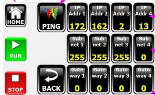
Sets the four octets of system IP Addresses from 0 to 255.
